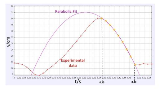
**Figure 5.** Experimental data for position versus time of the tail of the skateboard. Between t = 0.35 s and t = 0.48 s, a parabolic curve of equation  $y(t) = -12.08t^2 + 6.89 t - 0.42 (m)$  fits data quite well, indicating a movement with a constant acceleration of about 24.2 m s<sup>-2</sup>, considerably greater than the gravitational acceleration.
