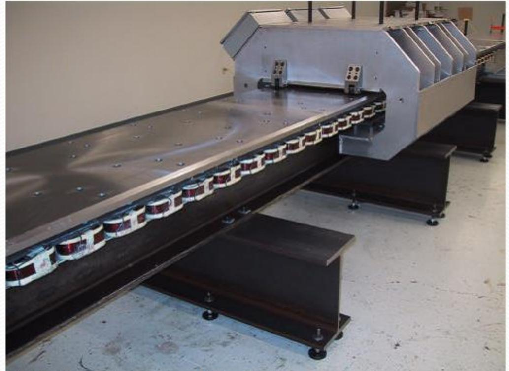
*Fig. 9.1. Photograph of prototype vehicle and guideway.*
